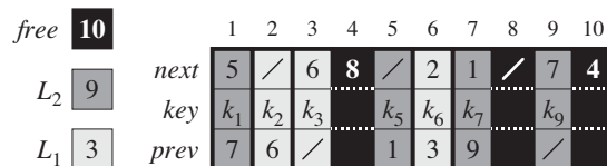
Figure 10.8 Two linked lists, L_1 (lightly shaded) and L_2 (heavily shaded), and a free list (darkened) intertwined.
